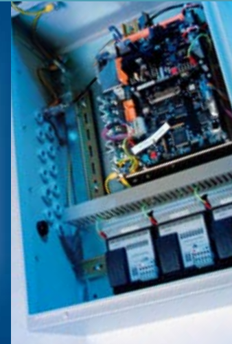
TSX24.3 telemetry station with built-in accumulator, 3 off expansion modules and radio with over-voltage protection.
