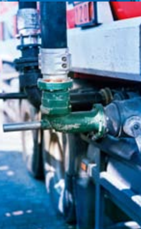
Top loading becomes replaced by bottom loading which is more efficient, safe and environmentally friendly.
