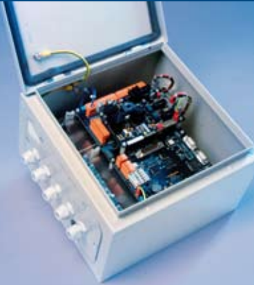
TSX24.1 is a compact telemetry station with GSM module and accumulator built-in.
